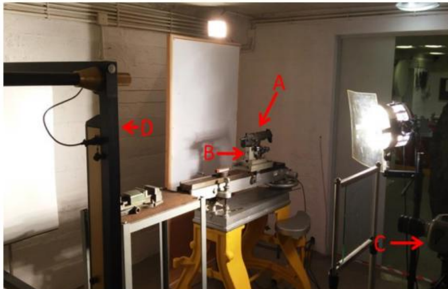
Fig. 3. Experimental set – up (A – investigated pistol, B – ballistic mount, C – high speed camera, D – precision light screen B-470)
