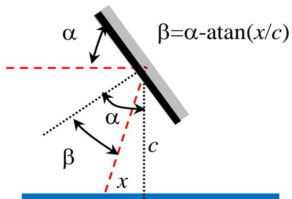
**Figure 2:**Ricochet Angles on Orthogonal Axis System
