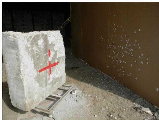
**Figure 3:**Material deflected from concrete target on witness panel
