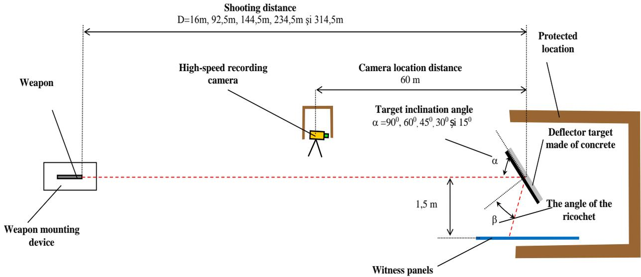
**Figure 1:**Testing Configuration Schematic
