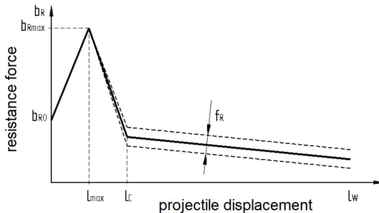
**Figure 3.** Dependence of barrel resistance force as the function of projectile displacement [2].
