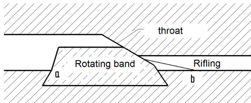
**Figure 1.** Scheme of rotating band – barrel elements configuration at the beginning of the engraving process.
