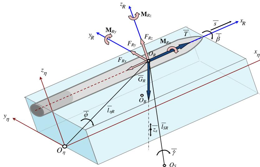
**Figure 3:** Applied forces and momentum on the unguided missile on a LAROM launcher
