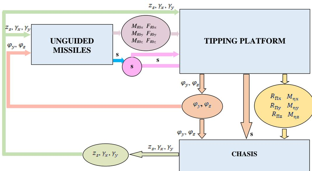
**Figure 6:** LAROM launcher parameters for MATLAB program
