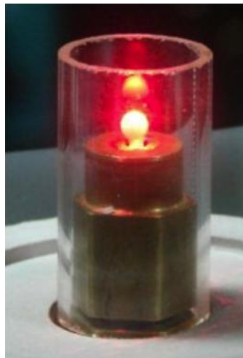
Figure 2. The copper jet with the spherical bead just before melting [2].
