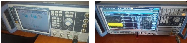
Figure 1. Signal generator (left) and signal analyzer (right)
