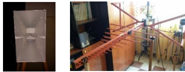
Figure 2. Transmitting (left) and receiving (right) antennas
