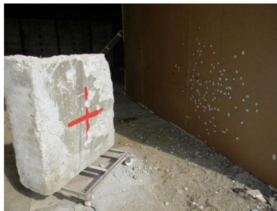
Figure 3: Material deflected from concrete target on witness panel
