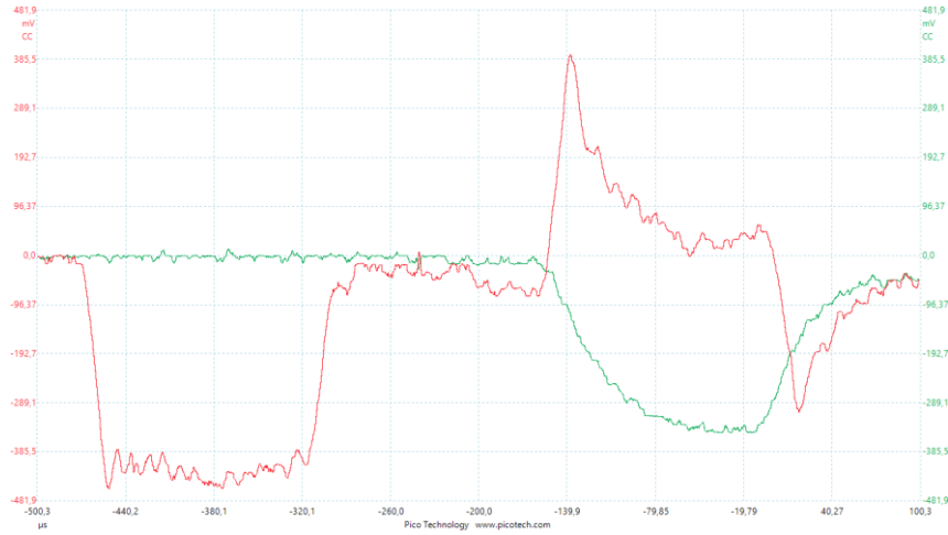
Fig.3 Signal acquired by oscilloscope during the SHPB test were the sample preserves its integrity
